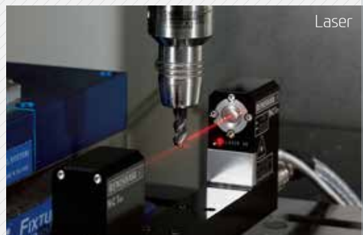
Automatic Tool Broken Detection Automatically detects breakage of tools.
